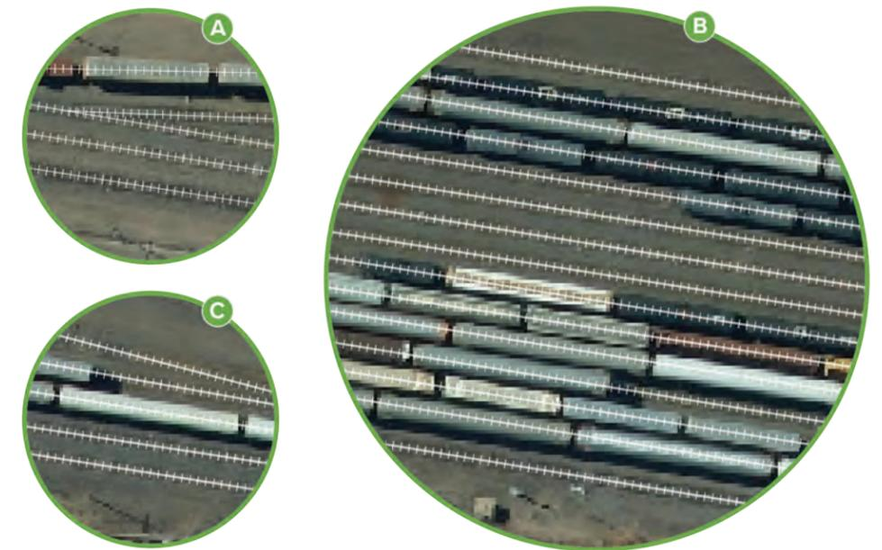
Up to 15 rail sidings occur in the area between San Jose Avenue and Smith Avenue where car consists are routinely stored, rearranged, and moved to transload facilities south of Woodward Road.
