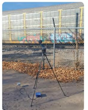
Sound level data was collected using a sound level meter.
