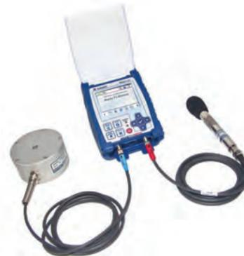
*Vibration data was collected using an InstanTel Micromate. Photo courtesy of Specto Technology.*
