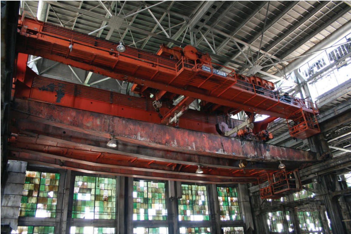
Machine Shop, Bay #4, Main 250 ton crane.
