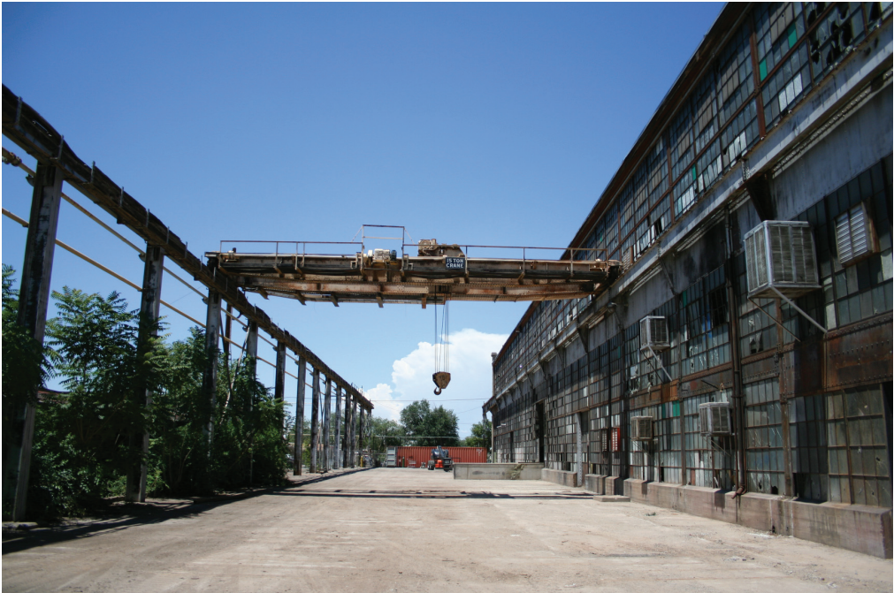
15 Ton Bridge Crane Connected to South Elevation of Machine Shop.
