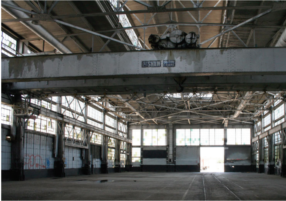
Tank Shop, Interior view, central bay with Shaw 30-ton crane in foreground.
