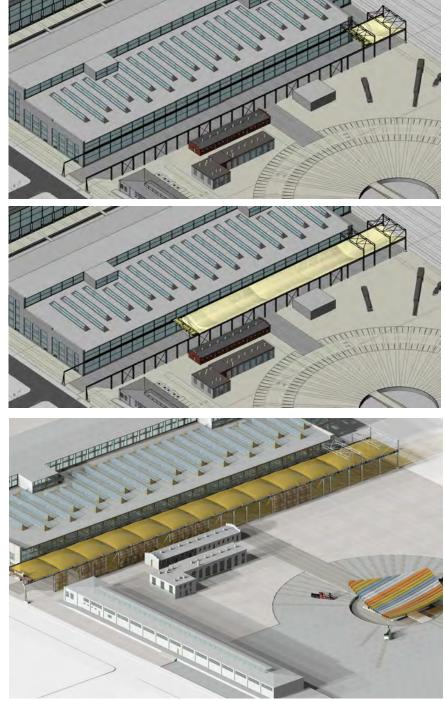
Phase 1 Concept showing Bridge Crane canopy operation
