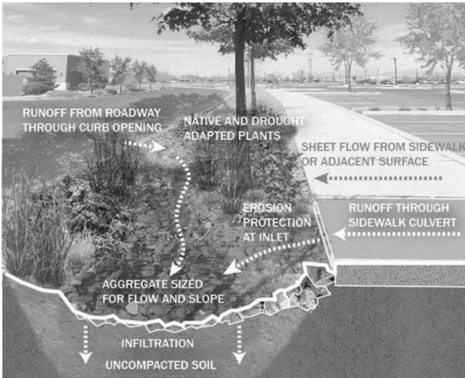
Stormwater Bumpout Diagram
