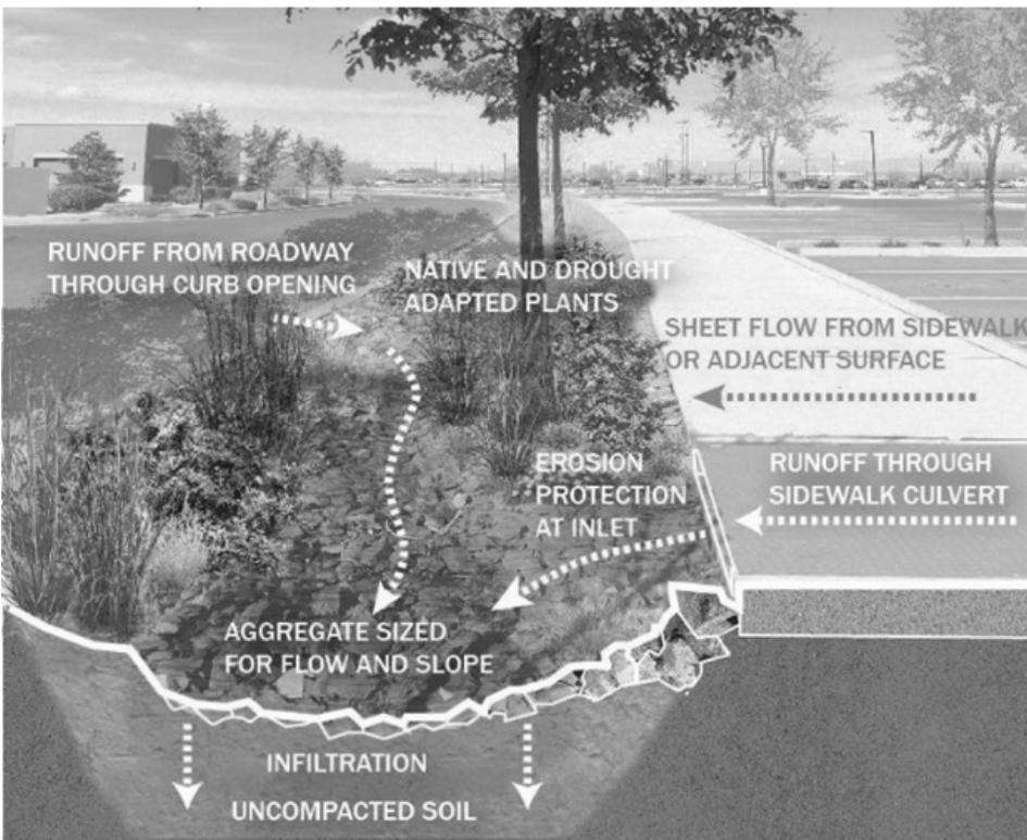
Stormwater Bumpout Diagram
