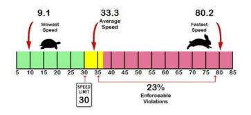
Speed Enforcement Evaluator Closest Cross Street **Total Percentage of Enforceable Violations GPS** 30 MPH 5 MPH Greater than 35 MPH Posted Speed Limit Enforcement Tolerance Latitude: 0.000000 Longitude: 0.000000 Enforcement Limit 50 **Analysis Dates** Start: 1/22/2021 End: 1/22/2021 **ADT** 5129 Combined
