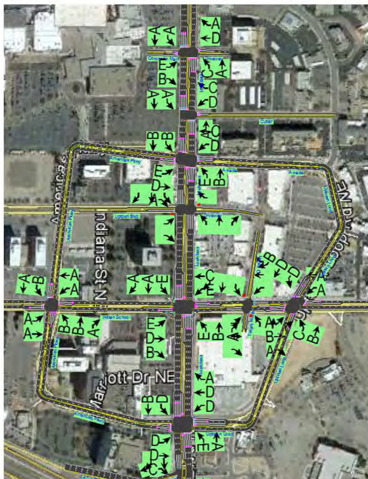
Figure 38. Current Year Noon Peak Hour Movement Level of Service – Existing Conditions (left) and With Recommendations (right)
