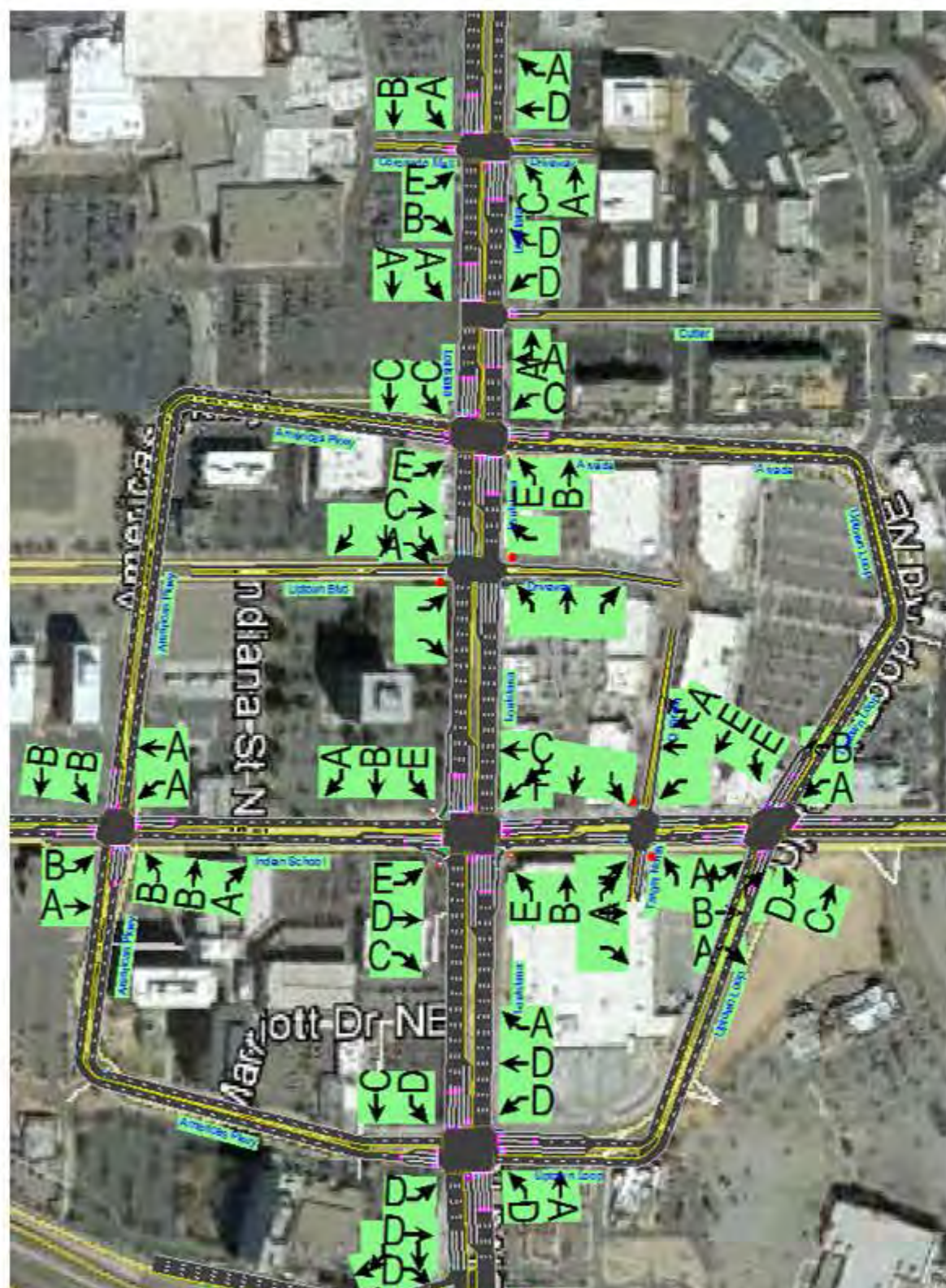
Figure 40. Current Year Friday PM Peak Hour Movement Level of Service – Existing Conditions (left) and With Recommendations (right)
