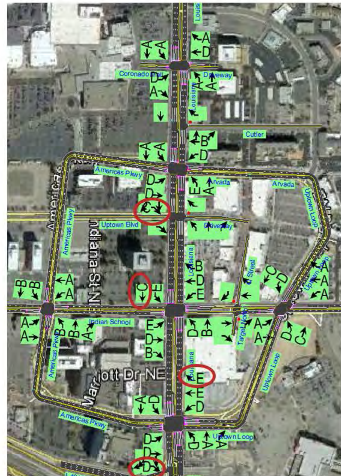
Figure 37. Current Year AM Peak Hour Movement Level of Service – Existing Conditions (left) and With Recommendations (right)
