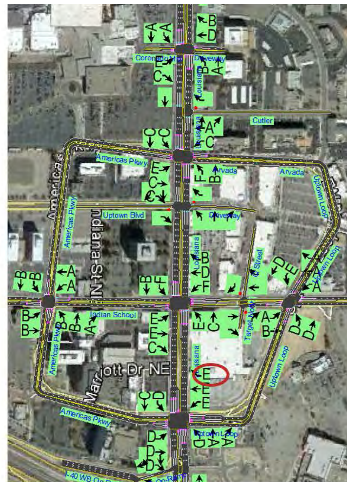
Figure 39. Current Year PM Peak Hour Movement Level of Service – Existing Conditions (left) and With Recommendations (right)
