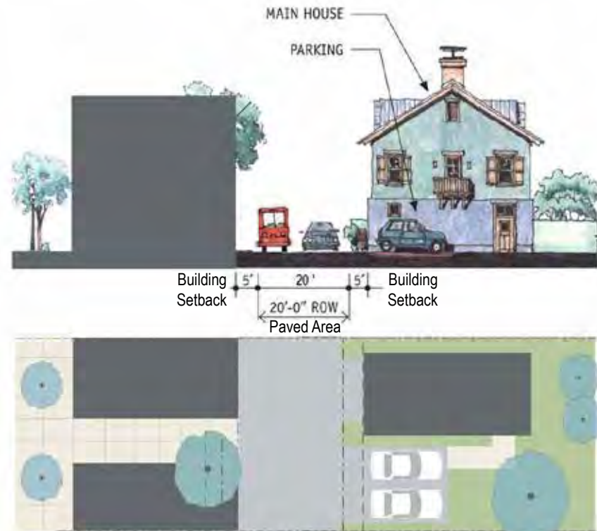
Exhibit 10.23 – Typical Commercial Alley Cross Section
