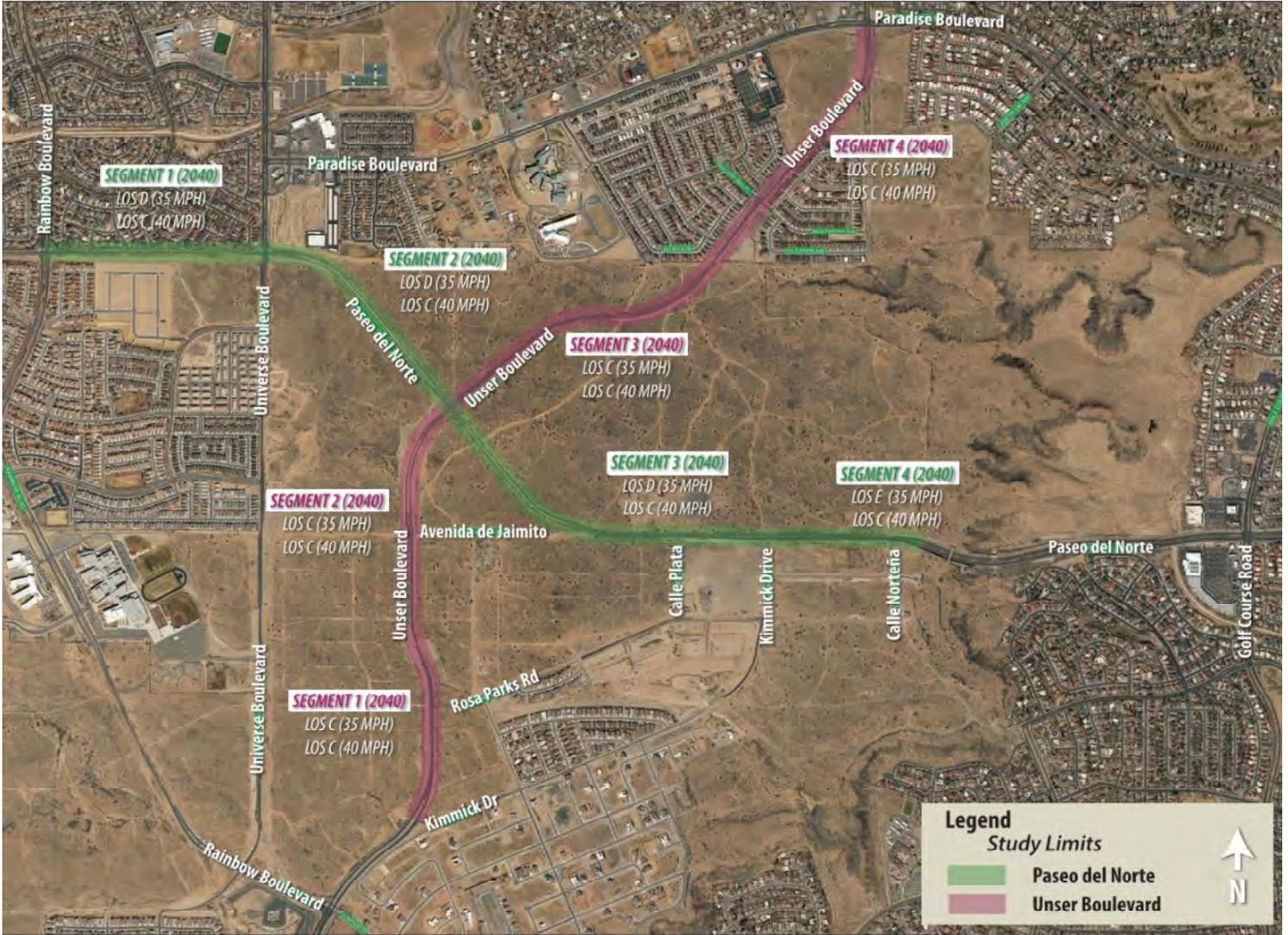
Figure 13: 2040 Estimated LOS – 35 mph and 40 mph Posted Speed
