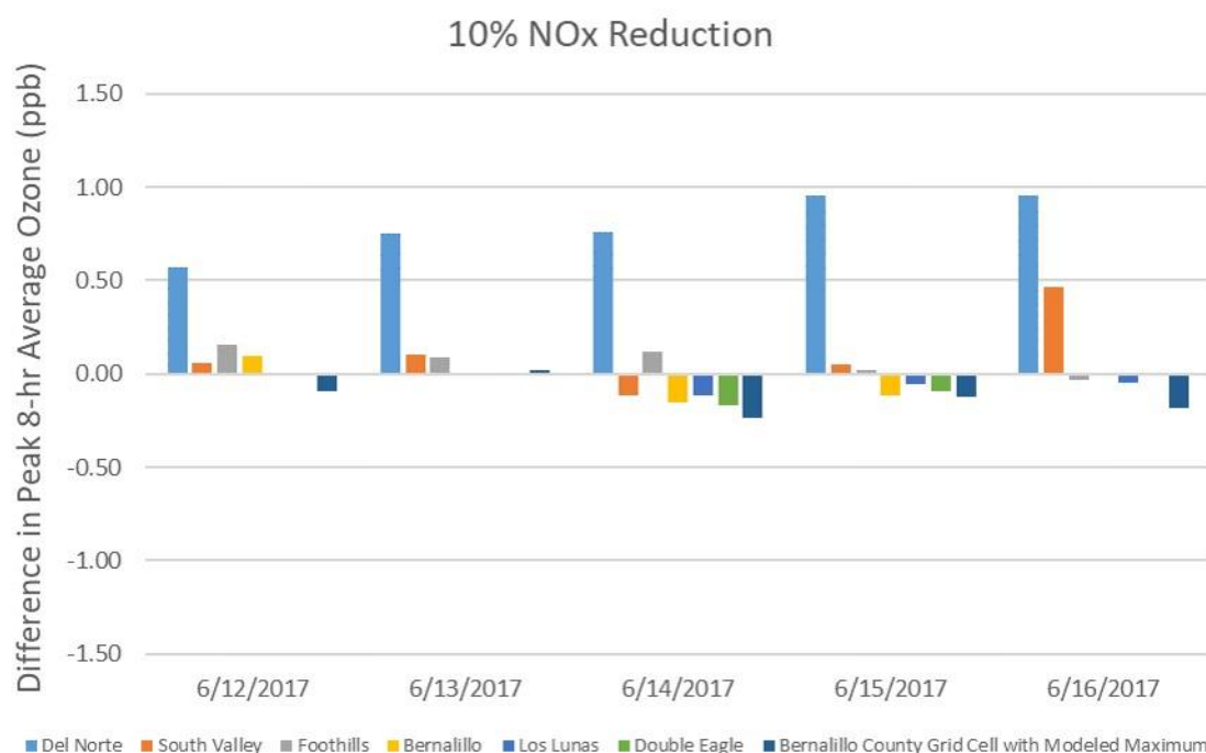
Figure 84. Differences in peak 8-hr average ozone concentrations between the 10% NO x reduction sensitivity simulation and the base-case simulation in the June ozone episode at the Albuquerque MSA sites, and at the grid cell where the highest ozone concentration was modeled in the base-case simulation (Bernalillo County Grid Cell with Modeled Maximum).
