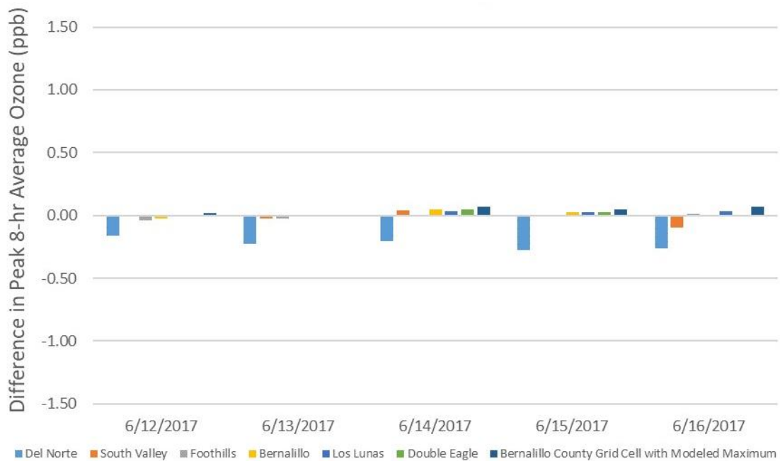
Figure 92. Differences in peak 8-hr average ozone concentrations between the I&M program sensitivity simulation and the base-case simulation in the June ozone episode at the Albuquerque MSA sites, and at the grid cell where the highest ozone concentration was modeled in the base-case simulation (Bernalillo County Grid Cell with Modeled Maximum).
