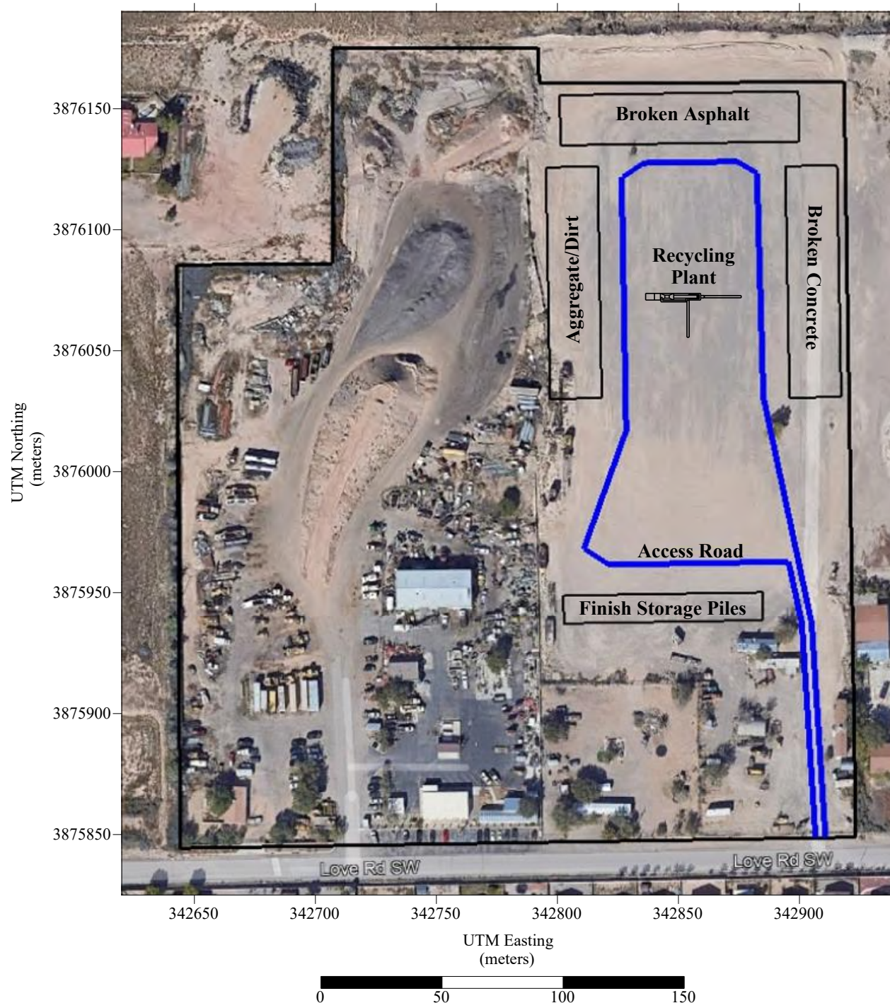
Figure 1: Star Paving's Love Rd Recycle Plant CBP Site Overview
