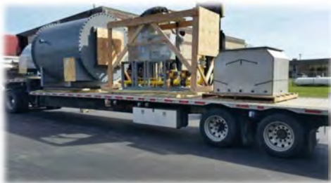
Figure 3-4. Thar/Dayco Supplied 11.7 MWt Natural Gas Fired Burner/Blower
