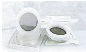
5. Put the assembled filter mount into a clean plastic bag to transport to the monitor site.
