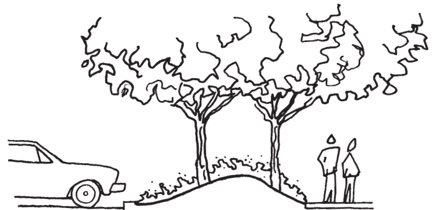
Screen parking lots with one or a combination of plant materials, walls, or berms.
