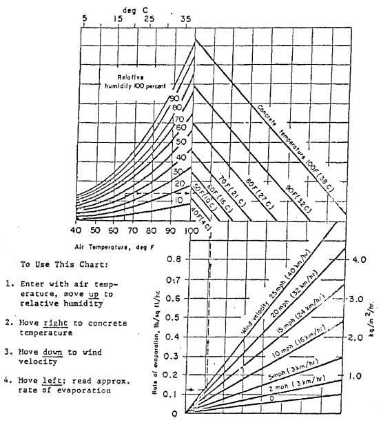
Effect of concrete and air temperatures, relative humidity, and wind velocity on the rate of evaporation of surface moisture from concrete. This chart provides a graphic method of estimating the loss of surface moisture for various weather conditions. To use the chart, follow the four steps outlined above. If the rate of evaporation approaches 0.2 lb per sq ft per hr (1.0 kg/m²/hr), precautions against plastic shrinkage cracking are necessary.
