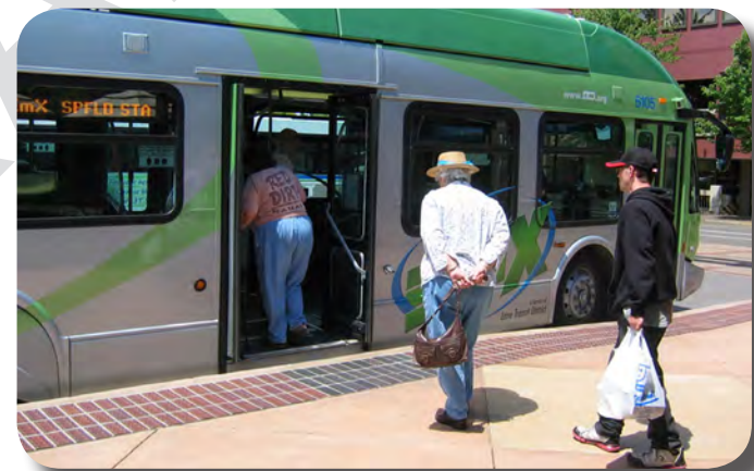
Example of a BRT vehicle at a level-boarding platform in Eugene, Oregon
