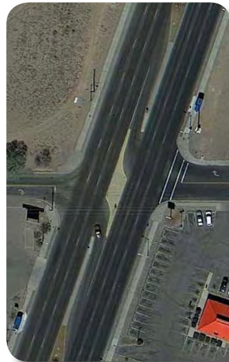
Example of a partial-access median opening
