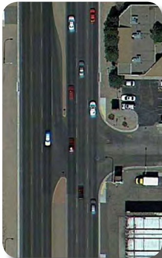
Example of a full-access median opening
