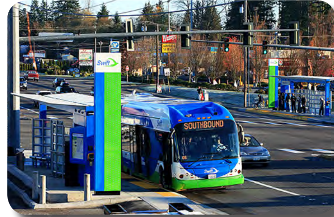
Example of a curbside-running BRT lane at a station in Everett, Washington
