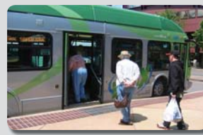
Example of a BRT vehicle at a level-boarding platform in Eugene, Oregon
