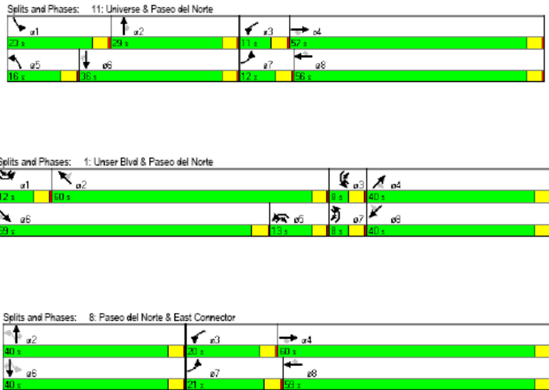
Figure 2-7 Signal Timing Concept: Planned Intersections
