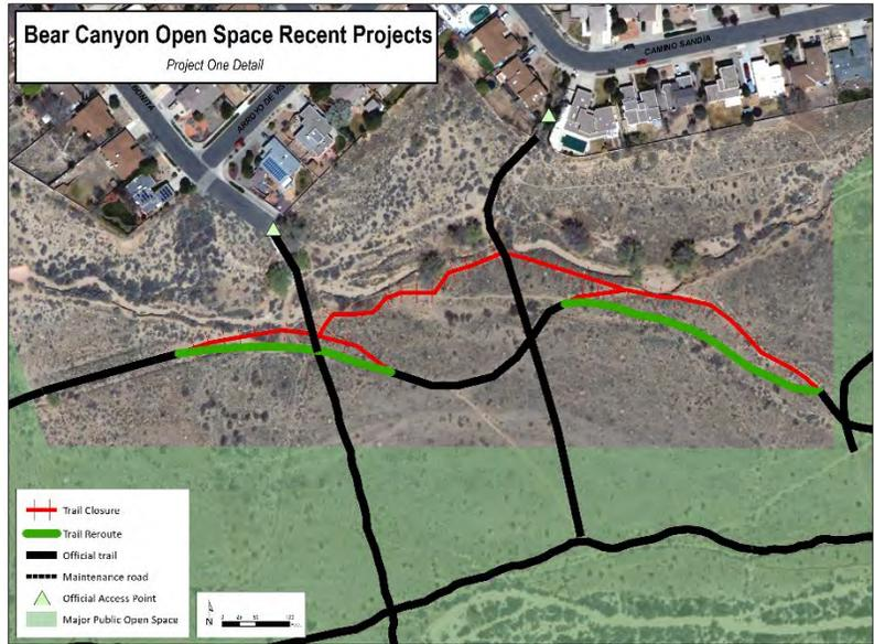
2. The OSD worked with ACE Charter School in 2018 to close and reroute additional sections of official trail in BCW that had partially collapsed into the drainage channel during a heavy rain event. The OSD did additional cactus plantings in 2019 to increase vegetation coverage and prevent usage of the closed section.
