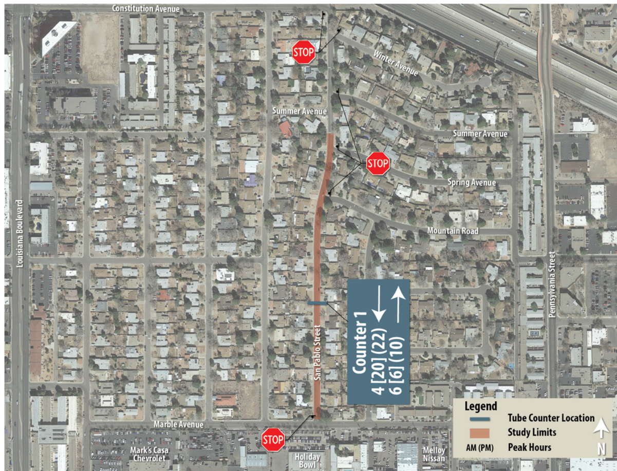
Figure 1: Project Area and Existing Traffic Volumes
