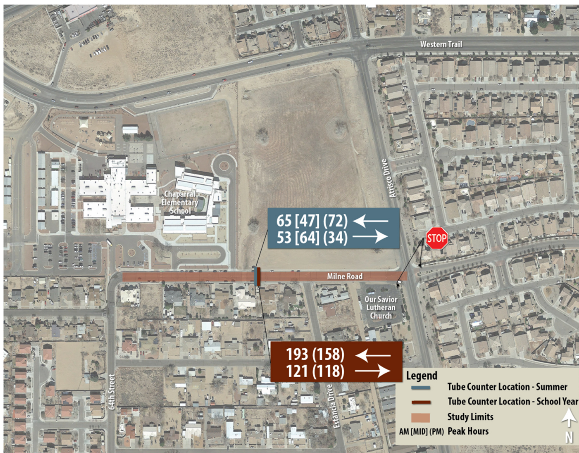
Figure 1: Project Area and Existing Traffic Volumes
