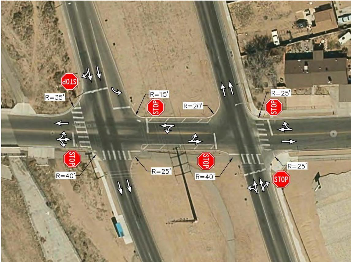
**Figure 3 – Intersection Control and Curb Return Radii**
