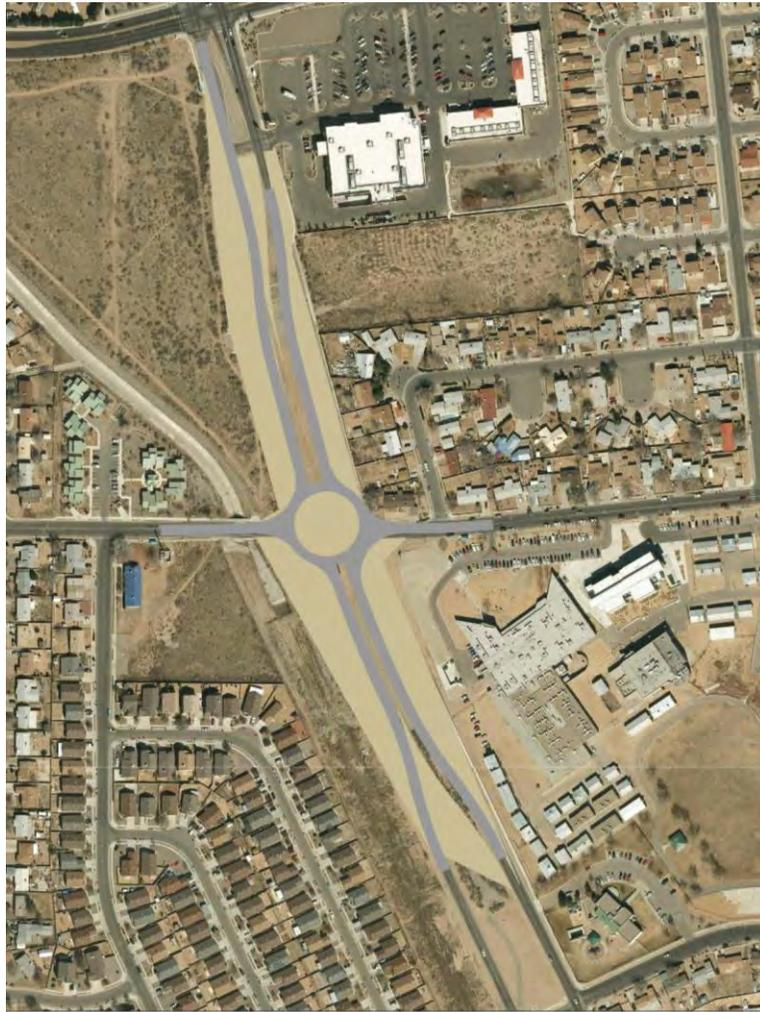
**Figure 22 – Roundabout Footprint**
