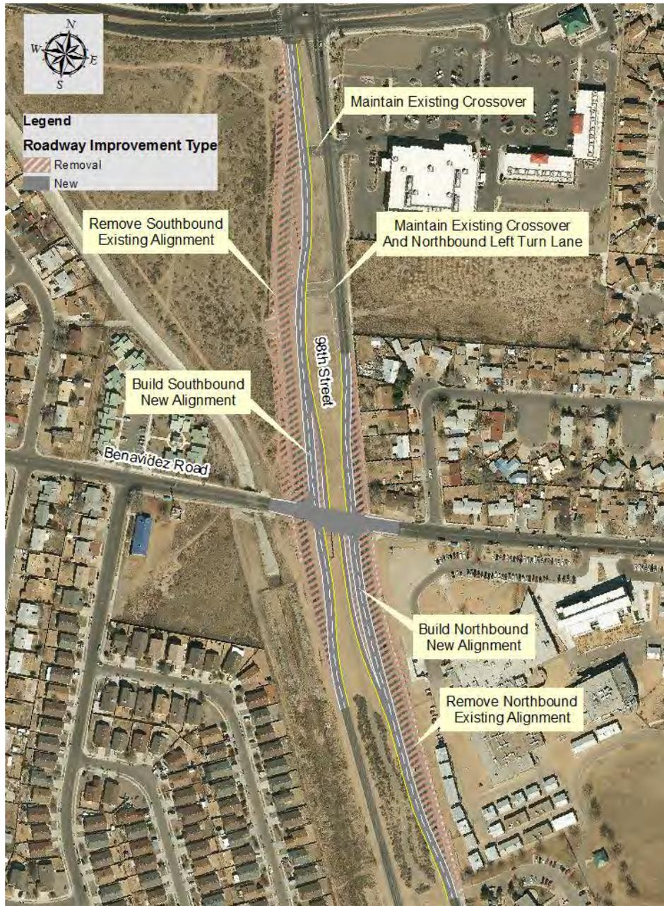
**Figure 15 – Realignment of 98<sup>th</sup> Street for Single Point Intersection**
