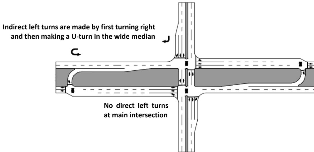
Figure 18 – Indirect Left Typical Lane Configuration
