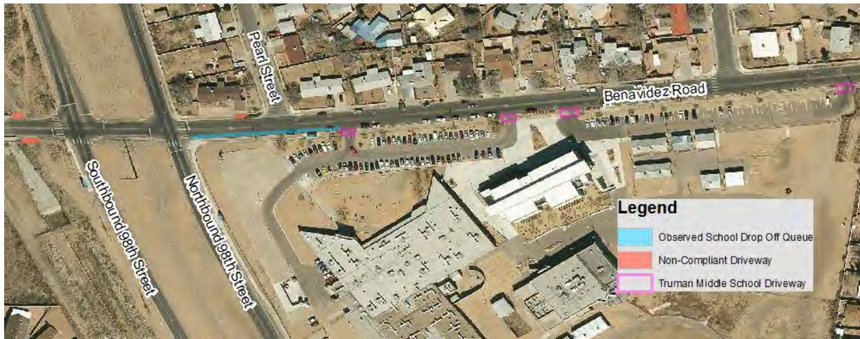
**Figure 4 – Driveways Based on Proximity to the Intersection**
