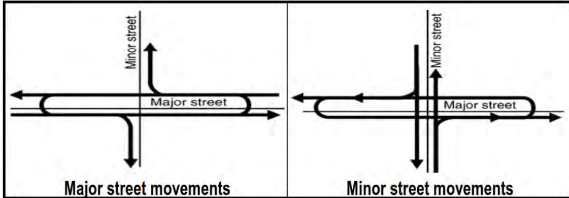
Figure 17 – Vehicle Movements through Indirect Left Treatment
