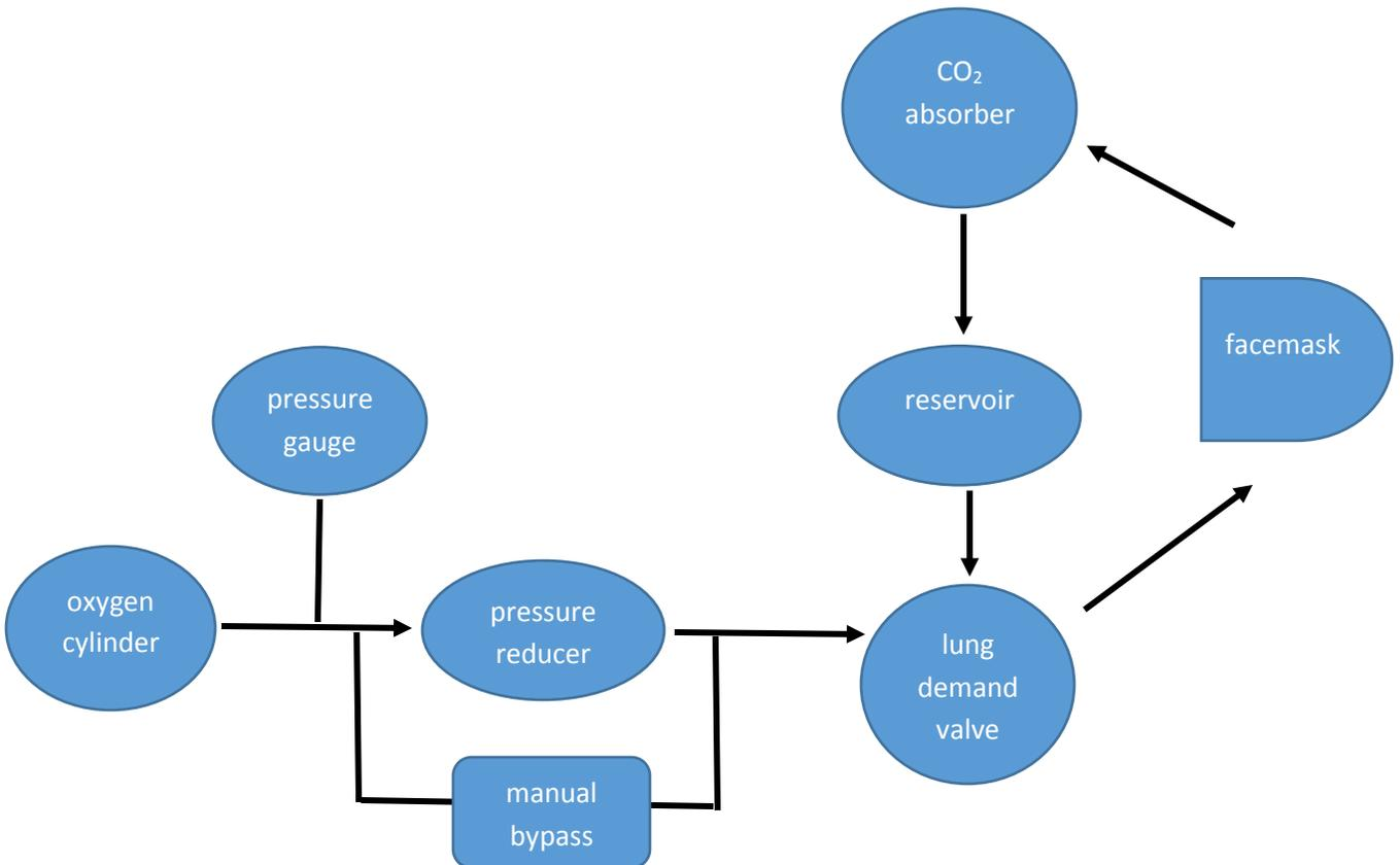
10. After leaving the facemask, oxygen must go through the \_\_\_\_\_ to reach the reservoir.
