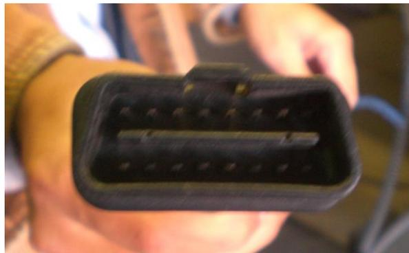
Figure 3 OBDII - Connector
