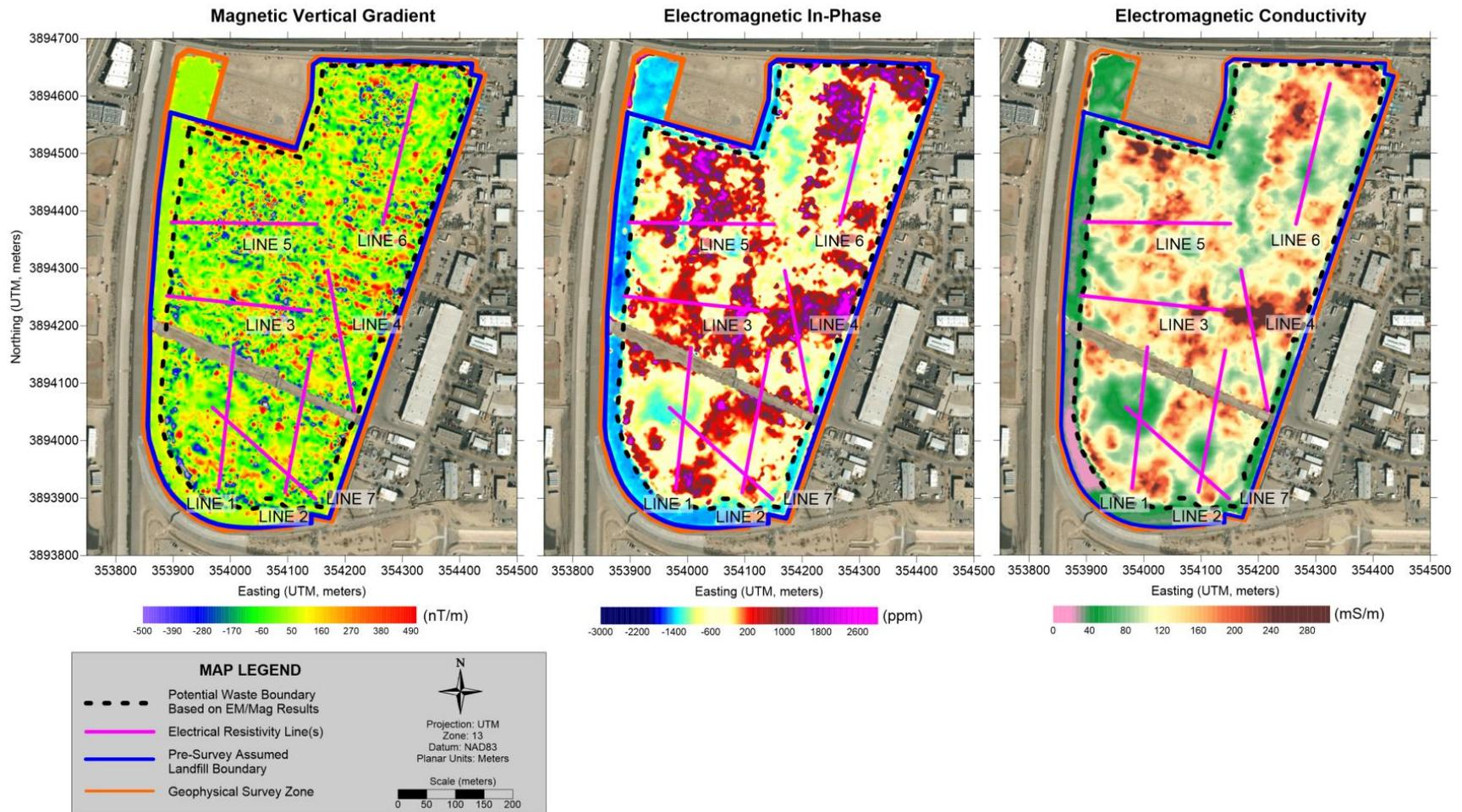
Figure 5. Magnetic Vertical Gradient Contour Map
