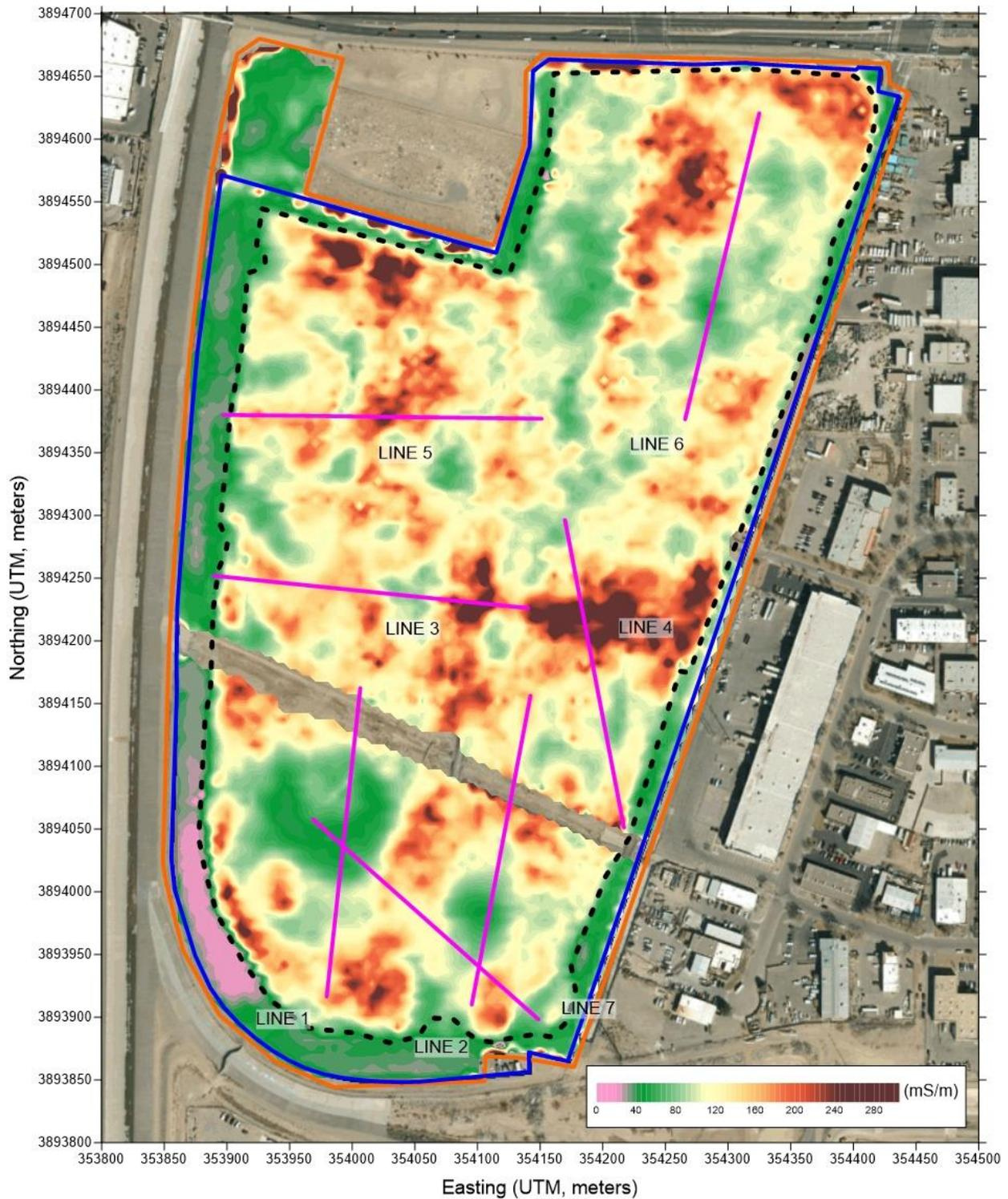
Figure 7. Electromagnetic In-phase Contour Map
