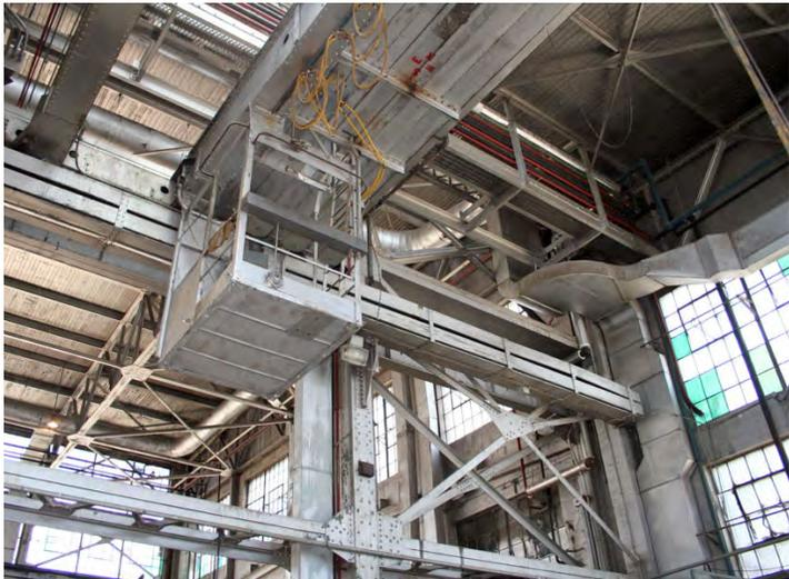
*Crane operator workstation, Heavy Equipment Bay.*
