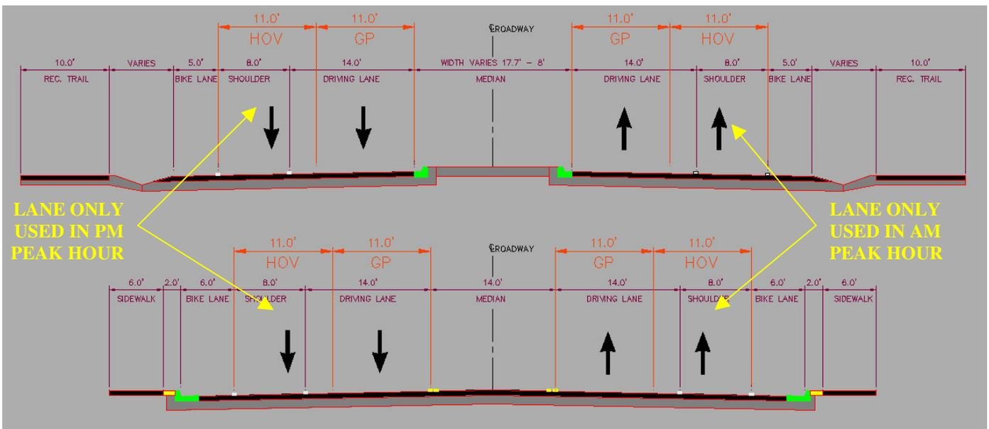
**Exhibit 14D – Montañó Road Typical Roadway Section with 1 Outside HOV Lane (AM/PM Peak Only) with 2 Inside General Purpose Lanes**
