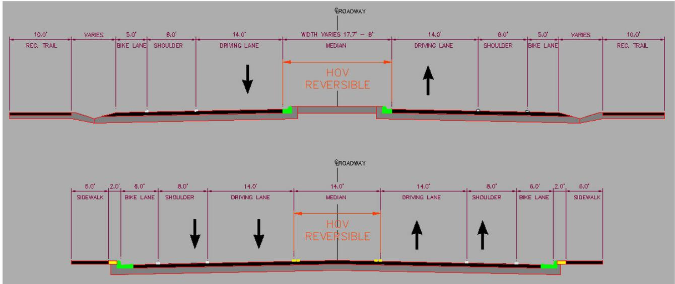
**Exhibit 14E – Montañó Road Typical Roadway Section with 1 Center (Median) HOV Lane with 2 General Purpose Lanes**
