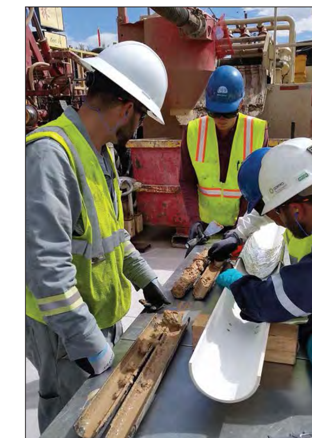
Looking at split spoon for lithologic description
