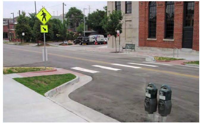
Figure 4.3.4. Example of a bump out and crosswalk
