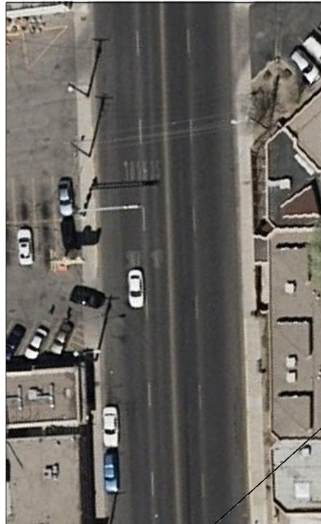
Typical Existing Lane Configuration (Without Left Turn Lanes)
