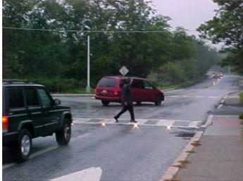
The pedestrian crossings are poorly marked at the intersection as a result of deteriorated pavement striping. A combination of restriping each crosswalk and pedestrian activated in-pavement flashing lights should be implemented to better mark the crosswalks for pedestrians. The in-pavement markings would be manually actuated through the pedestrian push buttons at each mastarm and would better define the crosswalk when in use. Stop bars at the intersection should also be refreshed.
