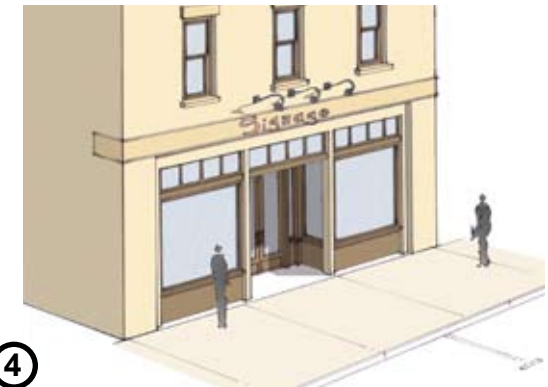
③ Columns sub-divide the shopfront opening
