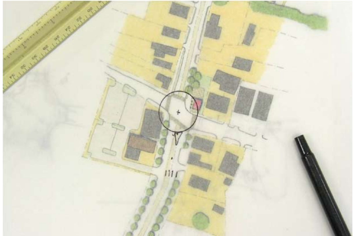
Figure 21: The inside of the circle drawn at the intersection at Griegos Road is what would be needed for a roundabout at this location. This would drastically impact properties and buildings on all four corners.
