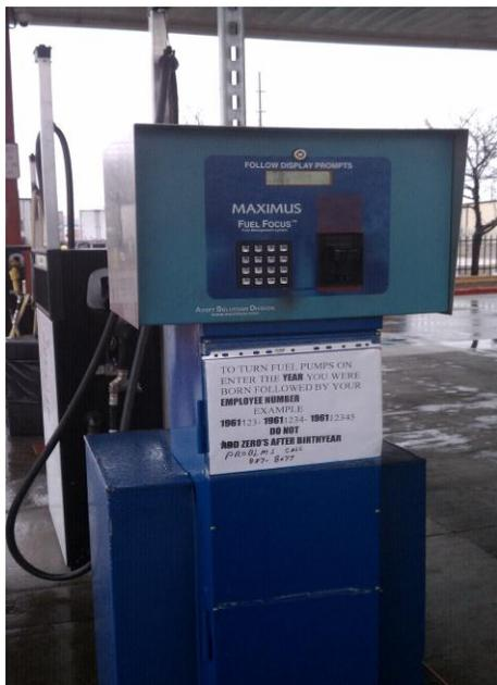
pump number, and a unique fuel pin number issued to them by FMD. FuelFocus will automatically recognize if any of the entered information does not agree with the information stored in the database and deny access for fuel.
